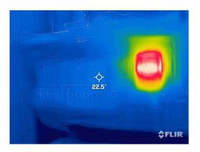
As you walk around your home, don't forget to look in hidden places such as inside cupboards, in the roofspace (if you have access), or the fuse box. This image shows the transformer for a front door bell that is no longer used as the owners now have a smart camera doorbell. However, the old transformer was left connected and is warm. It has been wasting power for years.
